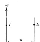
$$\begin{split} \vec{F}_{12} &= I_2 d \vec{\ell} \times \vec{B}_{12} = I_2 (-\hat{a}_z) \times \frac{\mu_0 I_1}{2\pi d} \hat{a}_\phi \\ &= \frac{\mu_0 I_1 I_2}{2\pi d} \hat{a}_r \ (排斥力) \end{split}$$
